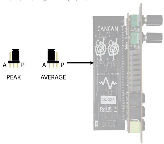
Reading the Meters – In Peak mode, the OdB indicator corresponds to a 10Vpp input signal level. The +3dB indicator corresponds to approximately 14Vpp, a high level that could cause clipping in subsequent stages. Aim for the OdB LED to illuminate for optimal levels. Note that the meter will show a lower level in Average mode since it doesn't respond to quick transient peaks.
