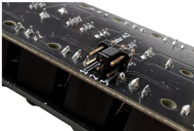
**NOTE:** It is possible to access these jumpers without removing the back PCB. But if you want to make it easier you can remove the back panel by unscrewing the 2 x M2 screws that connect the back PCB to the standoffs.
