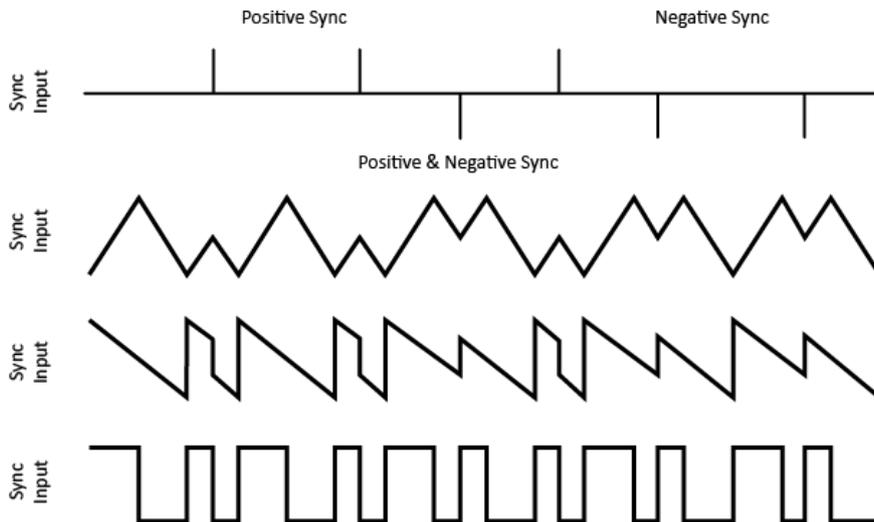
**SoftSync** - Negative pulses applied to the SoftSync input cause the upper peak to reverse direction prematurely, causing the oscillation period to be an integral multiple of the input sync pulse period. Avoid applying positive-edged pulse signals to the SoftSync input, as these manifest as transient spikes in the output waveforms.
