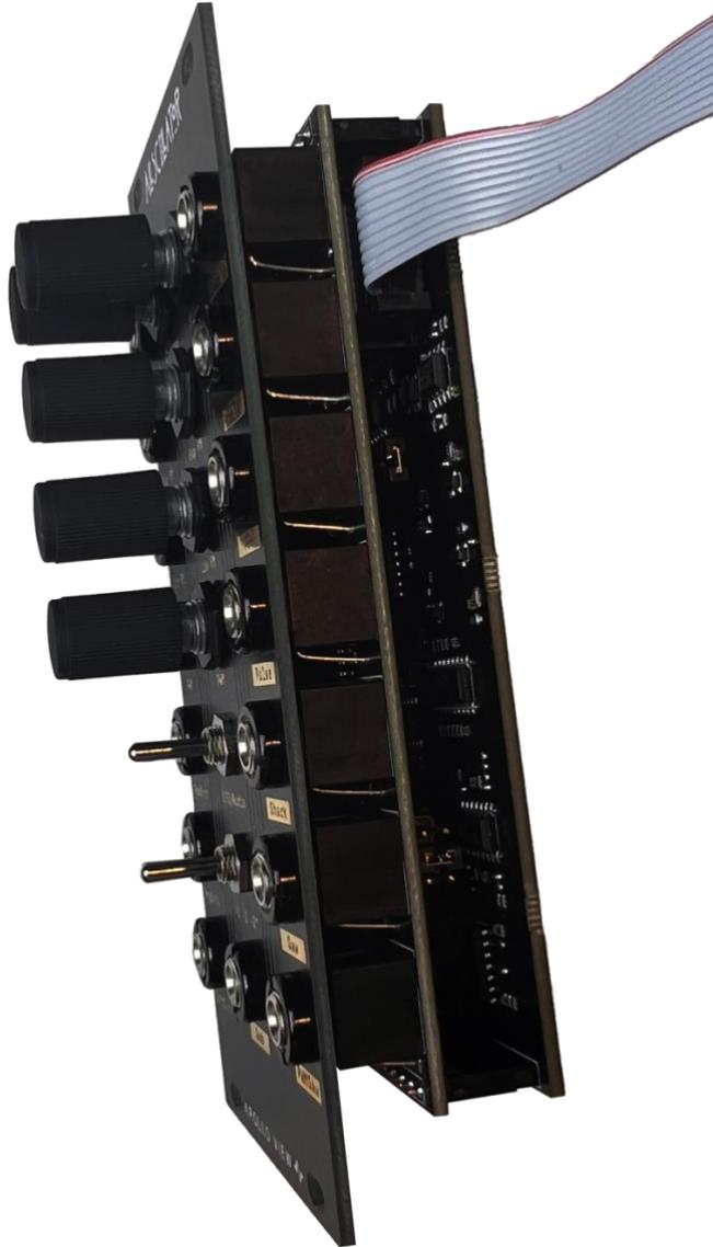
The module has reverse protection diodes, which will simply divert the reverse current to ground in case of incorrect installation.
