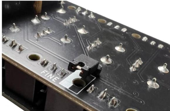
**LED Jumper** - The second jumper is situated directly behind the Saw output socket. The purpose of this jumper is to select the behaviour of the LEDs. It is possible to select the following behaviour with the position as indicated on the PCB silkscreen:
